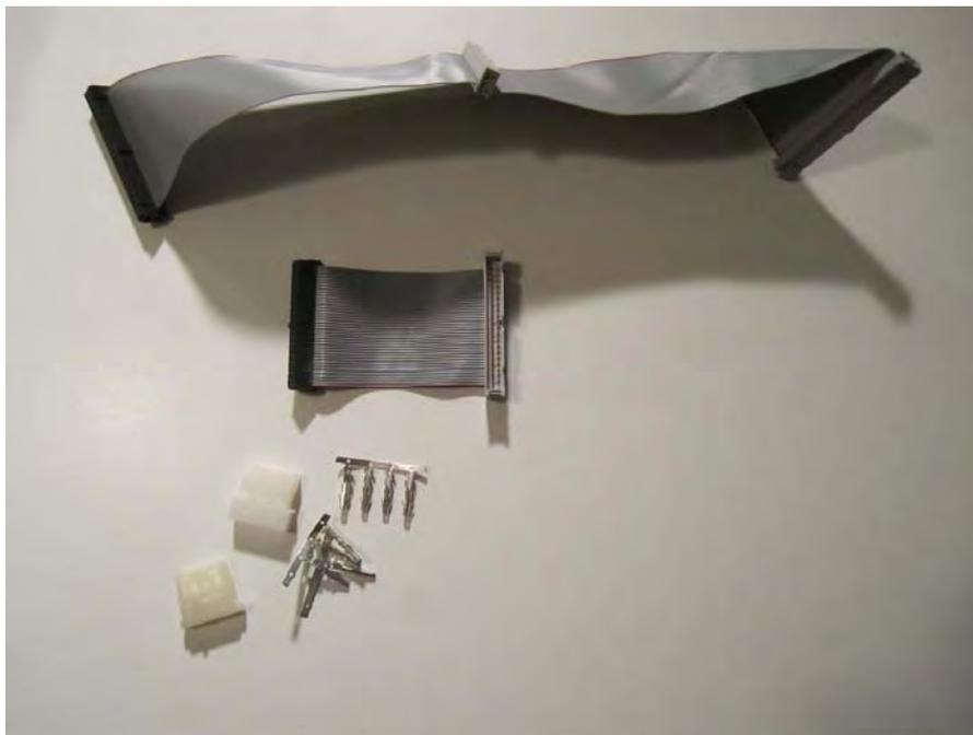
Cables are now cut and terminated. Note the IDE cable has one male end. The connector in the middle of the SCSI cable is not necessary – this was just a leftover from my other CF install. The white Molex connectors will be used to make a power cable extension.
