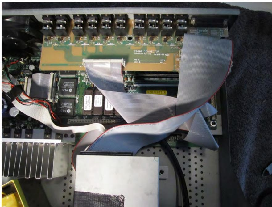
...and then plug the cable in backwards so that the red stripe (pin 1) of the cable is closest to the right side of the unit.
