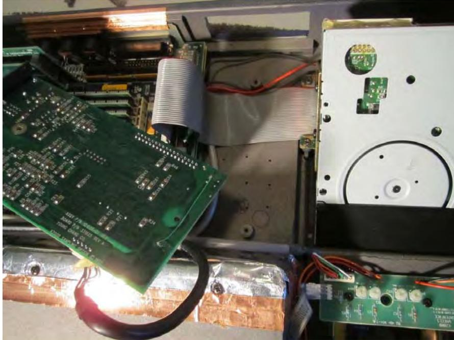
No need to unplug the SMP-K cables; just move the card out of the way to get to the FDD cables.
