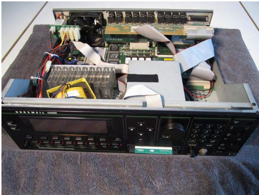
Remove the tape holding the display and button board ribbon cables onto the side of the drive bracket. Remove the four screws holding the bracket to the chassis (this will be self-explanatory once you start working). Do not remove the bracket and floppy drive yet.
