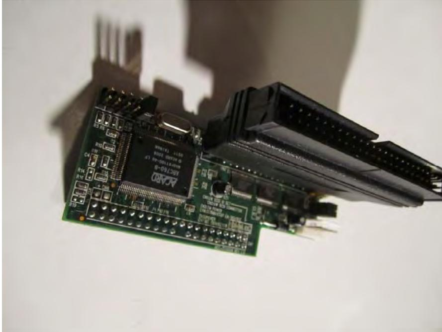
I used an AEC-7720UW and a 68 to 50 pin adapter with high byte termination. The AEC-7720U does not need an adapter.
