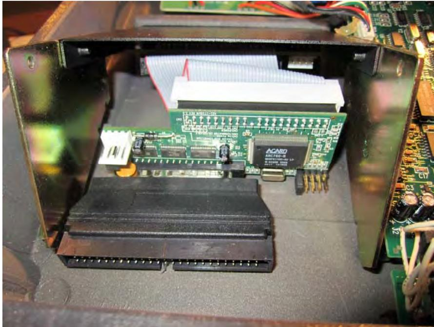
Attach the IDE cable between the drive and bridge. The good thing about using the adapter is that it provides a large enough surface to secure the assembly to the drive bay/top cover. I used hot glue for this, but you can also use double sided tape or Velcro. Leave enough room between the adapter and rear cover to insert/remove the SCSI cable.
