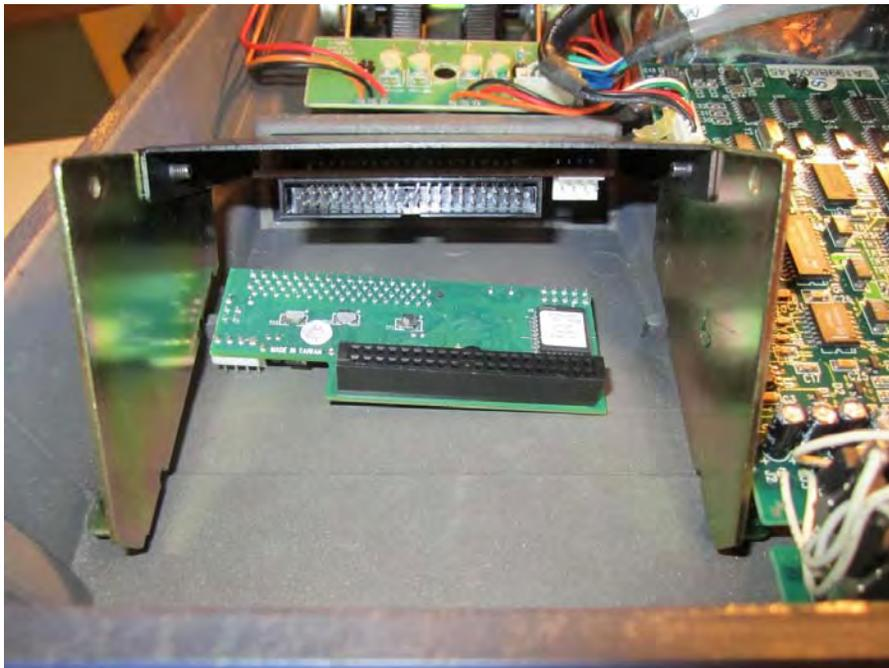
The reason we need a short male to female IDE cable is because the SCSI/IDE card would not clear the bracket if installed directly on the drive.
